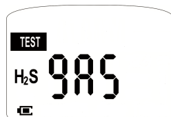
Figure 4-2: Manual Bump Test - Apply Gas
