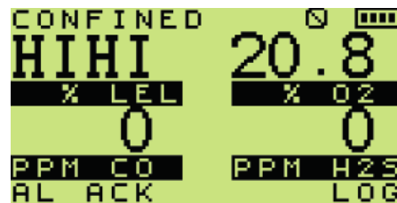
Figure 4-5: Confined Space Display (in alarm)
