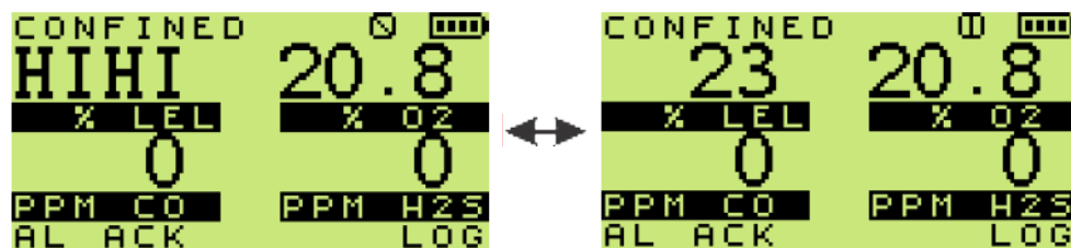
Figure 5-2: HIHI LEL Alarm
