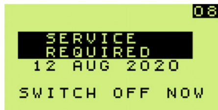
Figure 3-12: Service Due - Switch Off
