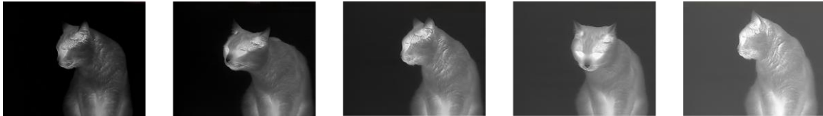
Figure 3-4 Adjust Brightness in White Hot Mode
