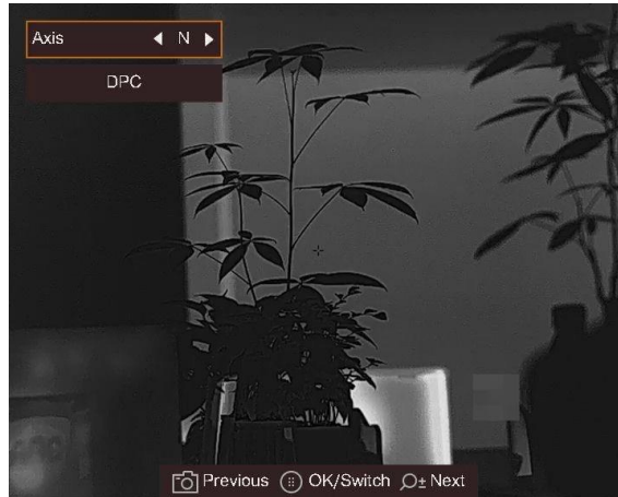
Figure 3-5 Correct Defective Pixel
