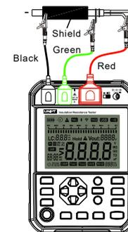
Fig. 10.1.3 Three-wire connection
