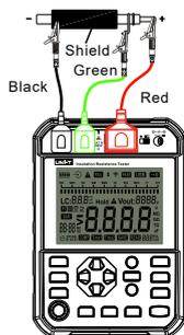
Fig. 10.1.2 Three-wire connection
