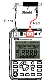
Fig. 10.1.1 Two-wire connection
