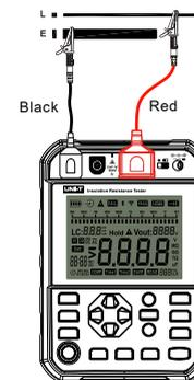
Fig. 9.3.2.1 Wire connection of voltage measurement
