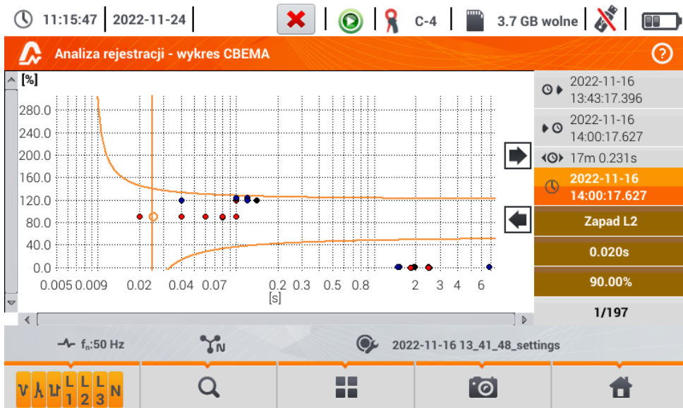
Fig. 5.27. Recording analysis – CBEMA graph
