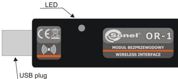
The OR-1 is used for wireless data transmission between a PC and SONEL S.A. meters equipped with a corresponding transceiver module. It provides a two-way communication.
