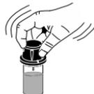
In order to avoid reagent leaking and to obtain more accurate measurements, close the cuvette first with the supplied HDPE plastic stopper
