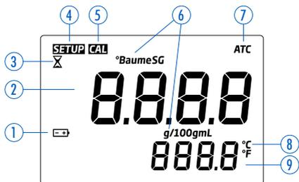
1. Battery (blinks when low battery condition detected)
