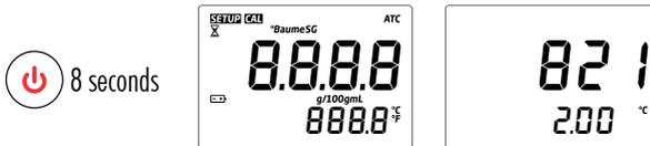
2. While continuing to hold the **ON/OFF** key, press the **ZERO** key. The temperature unit will change from °C to °F or vice versa.
