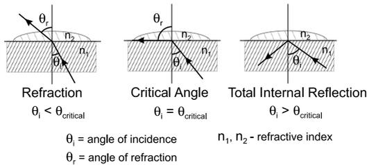
In the [HI96821](#), light from an LED passes through a prism in contact with the sample. An image sensor determines the critical angle at which the light is no longer refracted through the sample.
