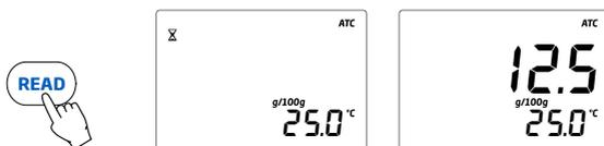
**Note:** The last measurement value will be displayed until the next sample is measured or the instrument is turned off. Temperature will be continuously updated.
