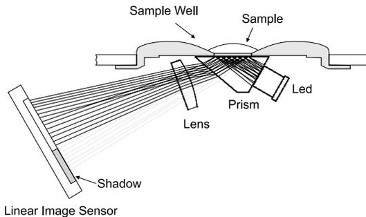
Specialized algorithms then apply temperature compensation to the measurement and convert the refractive index to: g/100 g (% by mass), g/100 mL, Specific Gravity (S.G. 20/20) or °Baumé.
