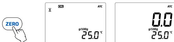
4. Gently absorb the ZERO water standard with a soft tissue. Use care not to scratch the prism surface. Dry the surface completely. The instrument is ready for sample measurement.
