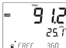
Pressing the **LOG** key again will stop the Interval logging session. The "LOG STOPPED" message will be displayed for a few seconds. If a sensor failure occurs during interval logging, the message "OUT OF SPEC." will alternate with logging information.
