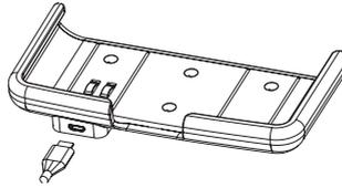
Connect the 3 mm probe jack to the socket located at the bottom of edge<sup>®</sup> D0. Slide edge<sup>®</sup> D0 into the wall cradle. Verify the battery icon indicates charging.
