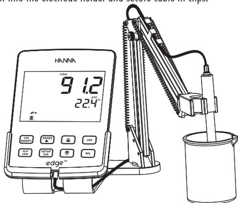
Connect the power adapter cable to the rear socket of the bench cradle. Connect the other end to the power adapter and plug into line power. Verify the battery icon indicates charging.
