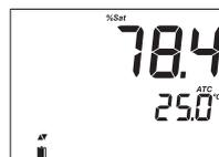
Press **RANGE/▶** key to change the reading from % to ppm (mg/L) and vice versa.
