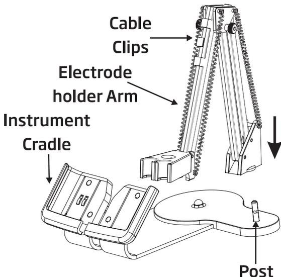
Slide **edge**<sup>®</sup> D0 into the cradle while positioning the probe cable behind the cradle. Put the probe/sensor into the electrode holder and secure cable in clips.
