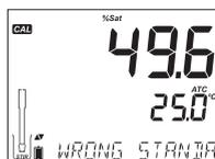
If the temperature is out of range (0.0 - 50.0 °C) during calibration, then the message “WRONG STANDARD TEMPERATURE” will be displayed and temperature value will blink.
