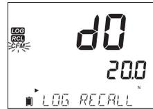
While the measurement type is blinking and message states “LOG RECALL”, press **SETUP/CLR** key.
