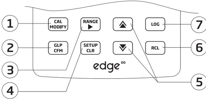
1. **CAL/MODIFY** - Used to enter and exit calibration mode. In SETUP, used to initiate changes of a configuration setting.
