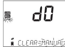
The lot number is used to identify particular sets of data. The lot numbers are allocated successively until 100, even if some lots were deleted. The total number of lots that can be saved is 100. If some are deleted (for example 1-50), fifty additional logs may be stored. These will be numbered 101-150. The lots are allocated successively (provided available memory space) until 999 is reached. After this, it is necessary to delete all the LOT logs to start over the numbering.
