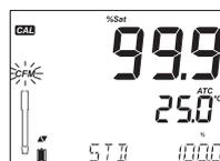
Press **CAL/MODIFY** key to leave calibration after the first point. The instrument will display “**SAVING**” message and it will return to measurement mode memorizing the slope calibration data.
