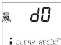
Press **GLP/CFM** key. The instrument will display “PLEASE WAIT” and then “CLEAR DONE” message. When individual logs are deleted within saved MANUAL or STABILITY logs, the logs will renumber, filling in the deleted data but staying in chronological order.
