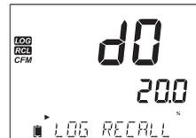
If no data was logged for the selected measurement range, the instrument displays the following messages:
