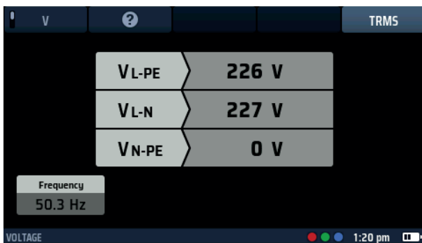
Fig 35: Voltage single phase
