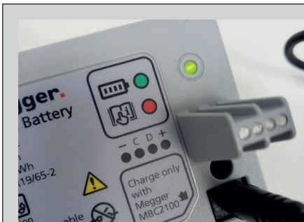
Fig 67: Battery pack connected
