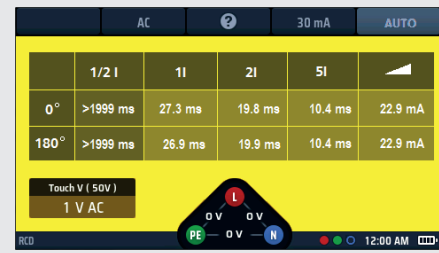
Fig 49: AUTO RCD test result progress
