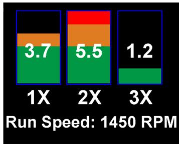
N.B. in order to perform a vibration analysis it is important that the running speed of the machine is entered correctly. This can be done with the “Setup Wizard” as described in Section 2.3.1 of this user guide, or by using the strobe attachment (see Section 5.1)
