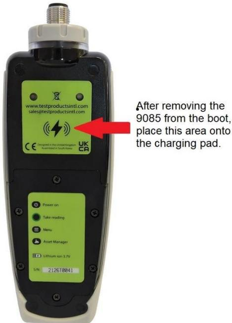
After removing the 9085 from the boot, place this area onto the charging pad.
