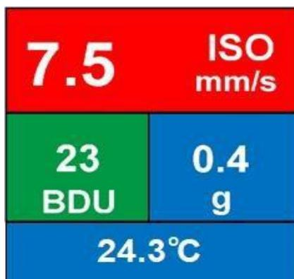
Taking a reading causes the overall vibration numbers and temperature screen to be displayed as shown in the example screen left.
