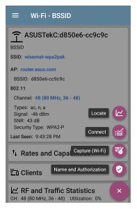
Tap Locate. This opens the Locate screen and causes your AirCheck G3 to "listen" for the BSSID or Client wireless devices you want to find using either the internal antennas or the optional external antenna (sold separately or in kits).
