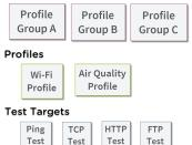
At the bottom level is a set of individual **Test Targets** that connect to network services, such as a web app or FTP site. A Test Target defines parameters including type, target URL/IP address, port number, and Pass/Fail thresholds. More complex tests, like HTTP, allow further Pass/Fail criteria, such as strings that must or must not be contained in the HTTP body. A Test Target can be added to and used in any number of **Profiles**.
