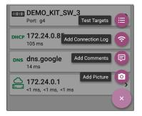
The Test Targets screen lists all of the defined and saved Test Targets. Checked boxes indicate the targets enabled in the current Profile. (Test Targets can be added to and used in any number of Wi-Fi Profiles.)
