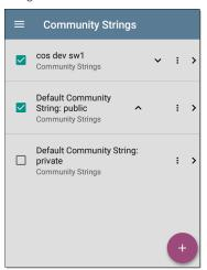
The LinkRunner uses the checked strings in the order shown on this screen. If it does not receive a response from the queried device using one string, it sends the next string.
