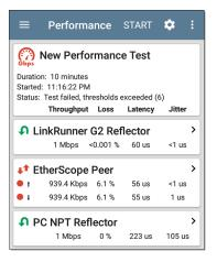
Performance results update every five seconds if you are using only Reflector endpoints, and/or an LinkRunner 10G Peer running v1.2 or newer software, with a test Duration of 4 hours or less. If you are running a 10 second test, all results display after 10 seconds. Otherwise, results update every 30 seconds.
