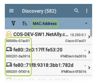
The selected Sort option displays in the Sort bar above the device list, and the sort characteristic for each device is shown under the device type icon. In the image above, all devices are sorted in order of the MAC Address.
