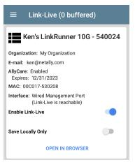
The LinkRunner unit's name that displays on the Link-Live.com is shown to the right of the Link-Live icon . You can change this name on the Link-Live.com Units . page.
