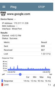
The graphs update in real time and then save and display data for up to 24 hours (depending on test type and/or link status).
