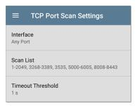
Interface: Tap the field to select the LinkRunner port from which the port scan runs. (See Selecting Ports for explanations of the different ports.)
