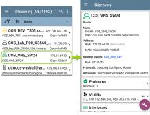
The available data and actions on the Details screens vary significantly depending on the device type, connections, and data the LinkRunner was able to discover. In other words, only the discoverable information for each device is shown on the Details screen.
