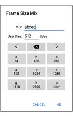
On the Frame Size Mix keyboard shown above, each letter (a through h) is associated with a frame size. The default pattern is "abceg," meaning the traffic pattern follow a repeating sequence of 64, 128, 256, 1024, and 1518 bytes. Use the letter keys along with the arrows and backspace button to edit the mix sequence as desired.
