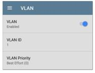
Tap to open the VLAN settings screen. Slide the toggle to the right to enable VLAN testing. Enabling this setting also enables a VLAN test card on the Wired AutoTest results screen. Once enabled, VLAN ID and VLAN Priority fields appear. Tap these fields to open a pop-up number pad and enter the correct ID and priority. Tap OK to save them.
