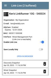
The buffered files displayed automatically upload to Link-Live.com once your LinkRunner connects to an active network
