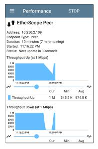
The Service results screen displays detailed test characteristics and graphs of performance.
