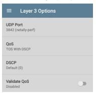
**UDP Port**: Tap to enter a specific UDP port number. This can help you simulate prioritized traffic on ports reserved for specific uses such as video, voice, or backup data or to match ports allowed by a firewall.
