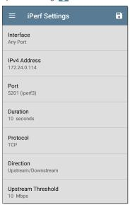
Tap each field to enter or revise selections as needed. Changed settings are automatically applied. When you finish configuring, tap the back button do to return to the iPerf test screen.
