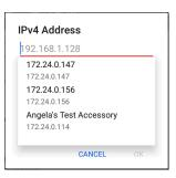
A drop-down list in the IPv4 Address dialog shows all the Test Accessories the LinkRunner has discovered through the discovery process, as well as any Test Accessories that are claimed to the same Link-Live organization as your LinkRunner.
