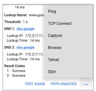
Tap blue links or the blue action overflow icon ... at the bottom of the test results screens to run the DNS Test Again, open another app
