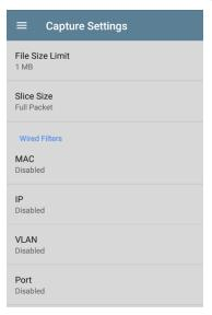
File Size Limit: Tap this field to specify a size for the capture file. The default size is 1 MB, and largest size allowed is 1000 MB. The capture stops when the captured file reaches this size.
