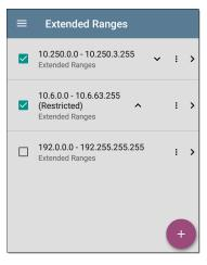
Check or uncheck the boxes to include or exclude an extended range from the current Discovery configuration. Unchecked Extended Ranges do not affect the default Discovery behavior in the current configuration, but they may be used in other Discovery configurations (like Community Strings and Credentials).
