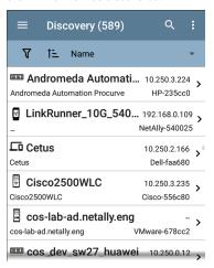
Like in AutoTest and other LinkRunner screens, the icons in Discovery change color to indicate a Warning or Failure condition. Discovery also displays device icons in Blue to indicate Problem-related information that does not constitute a warning or failure, and **Green** to indicate that a previous Problem has been resolved. (See the Problem Settings to adjust enabled Problems and thresholds.)
