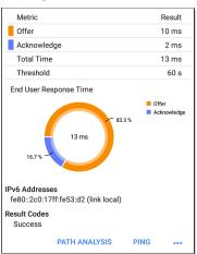
Offer: Time between when the LinkRunner sent the discovery and received an address offer from the DHCP server
