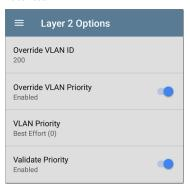
Override VLAN ID: Tap to select or enter a VLAN ID number. The Override VLAN ID function tags frames with a particular VLAN (for example, a VLAN used for voice, video, or data). If Override
