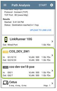
The LinkRunner is able to identify these Layer 2 switches and their interfaces because it has configured SNMP access to the switches.
