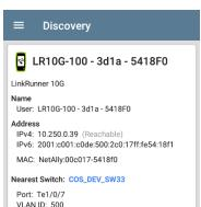
The Nearest Switch link opens a Discovery app Details screen for that device.
