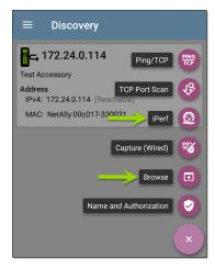
Select the iPerf app button to open the iPerf app with the IP address populated from the Test Accessory in Discovery.
