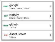
AutoTest Target tests are user-assignable endpoints to which LinkRunner 10G attempts to connect each time the AutoTest profile runs. These tests ensure availability of internal or external websites, servers, and devices to users of your network.
