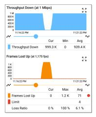
Touch and drag (or swipe) left and right on each graph to move backward and forward in time, and double tap or move the slider to zoom in and out. See the Trending Graphs topic for an overview of the graph's pan and zoom controls.
