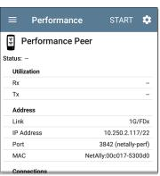
The Wired Test Port must be linked (by running an AutoTest Wired Profile) for the Performance Peer function to run. If the port is not linked, a Status message displays, "The wired test port is not linked."
