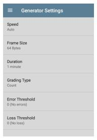
Tap each field to enter or revise selections as needed. Changed settings are automatically applied. When you finish configuring, tap **OK** or **Cancel** to return to the settings screen. When you finish configuring, tap the back button to return to the LANBERT test screen.
