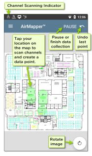
If you use the default Auto Sampling (Passive) survey, you can collect data points automatically, especially when sampling in straight lines such as long hallways or when crossing open spaces.
