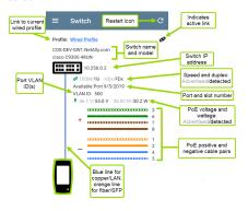
The main Switch screen has only a few controls and no settings.
