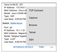
Tap TCP Connect to open the corresponding NetAlly apps, populated with the switch's address.
