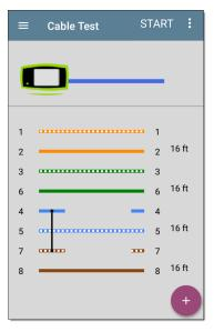
This unterminated cable test image shows a shorted cable between pins 4 and 7.
