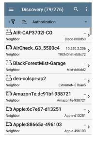
NOTE: Batch Authorization operates on the default MAC address of a device. If a device has multiple MACs, authorization is set only on the default MAC address. Devices that do not have a discovered MAC address, such as unknown switches and off-net devices, cannot have an authorization setting.
