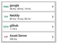
AutoTest Target tests are user-assignable endpoints to which LRAT 3000-4000 attempts to connect each time the AutoTest profile runs. These tests ensure availability of internal or external websites, servers, and devices to users of your network.
