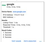
**Device Name:** Hostname or address of the target device.
