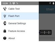
Tap Flash Port to open the Flash Port screen. If the connection to the switch is good, a blue line connects a test unit icon to a switch icon.
