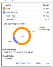
Offer: Time between when the LRAT sent the discovery and received an address offer from the DHCP server
