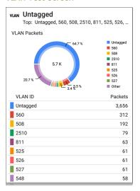
The VLAN test screen displays the real-time traffic the LRAT detects on the top VLANs. Up to nine VLANs with the highest traffic are displayed as colored portions of the pie chart. The table on
