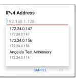
A drop-down list in the IPv4 Address dialog shows all the Test Accessories the LRAT has discovered through the discovery process, as well as any Test Accessories that are claimed to the same Link-Live organization as your LRAT.
