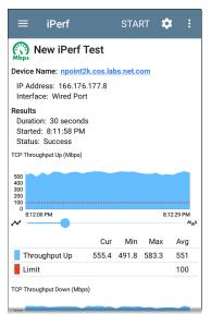
Test characteristics and status are displayed at the top of the iPerf results screen while the lower part of the screen displays a real-time graph of the TCP or UDP Upload and/or Download speeds. To pan and zoom on the graphs, you can swipe, double tap, and move the slider. See the Trending Graphs topic for an overview of the graph controls.
