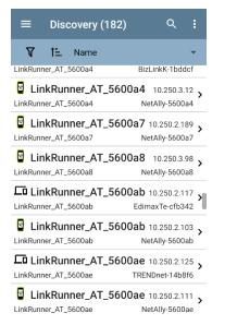
Like in AutoTest and other LRAT screens, the icons in Discovery change color to indicate a Warning or Failure condition. Discovery also displays device icons in Blue to indicate Problem-related information that does not constitute a warning or failure, and Green to indicate that a previous Problem has been resolved. (See the Problem Settings to adjust enabled Problems and thresholds.)
