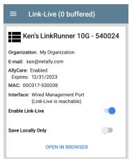
The LRAT unit's name that displays on the Link-Live.com is shown to the right of the Link-Live icon . You can change this name on the Link-Live.com Units . page.
