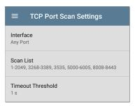
**Interface:** Tap the field to select the LRAT port from which the port scan runs. (See Selecting Ports for explanations of the different ports.)
