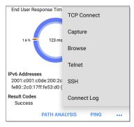
The additional actions available on the DHCP test screen include opening the Path Analysis, Ping/TCP, or Capture apps populated with the DHCP server address, browsing to the IPv4 address in the web browser, starting a Telnet or SSH session, or viewing the Connect Log.
