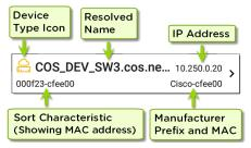
The lower left field displays the characteristic by which the Discovery list is currently sorted. In the image above, the list is sorted by MAC address. See Discovery Sorts in this topic for more about sorting.
