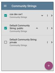
The LRAT uses the checked strings in the order shown on this screen. If it does not receive a
