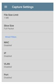
File Size Limit: Tap this field to specify a size for the capture file. The default size is 1 MB, and largest size allowed is 1 GB (1,024 MB). The capture stops when the captured file reaches this size. When capture is running, the capture screen displays the current file size as data is captured.
