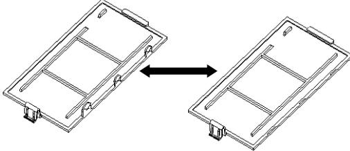
2. Install the Interface PCB. Push it through the pins and secure it with the 4 screws.
