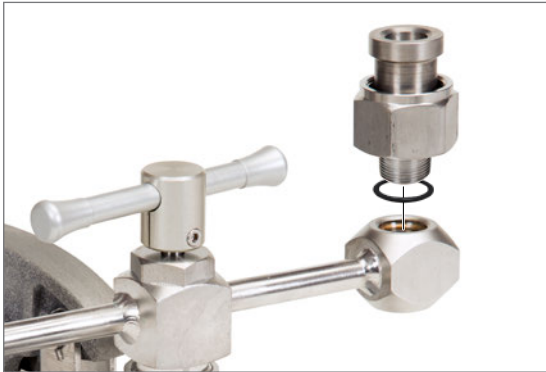
Remove the union nipple, nut, and o-ring...
