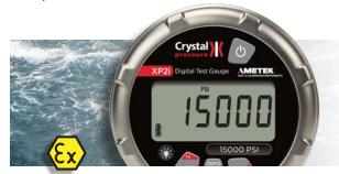
**Digital Test Gauge** The XP2i is an ultra-rugged digital test gauge with 0.1% of reading accuracy up to 15,000 psi/1000 bar. The ruggedized housing withstands vibration, a fall from up to 2 meters, and accidental overpressure at up to two times the indicated limit. Perfect for direct use in any Zone 0 hazardous area pressure application.
