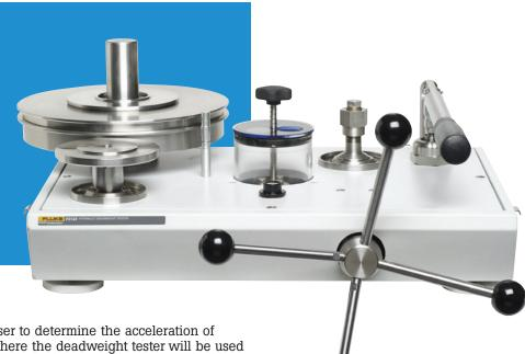
The most accurate method for the user to determine the acceleration of gravity at the laboratory or other site where the deadweight tester will be used is to have a site survey performed. There are various companies that can provide this type of service. Although this is the most accurate method, it can also be expensive.
