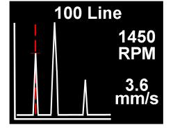
The readings to the right of the screen show the frequency (in Hz or RPM) and the RMS vibration level (in mm/s or inch/s) at the position of the cursor (red dotted line). The cursor position can be moved by use of the left (<) and right (>) arrow buttons.
