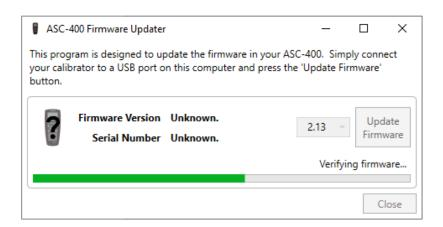
To complete the firmware update, remove AC adaptor and batteries from ASC-400.
