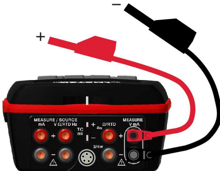
Figure 13 mA current measurement connection (upper window)
