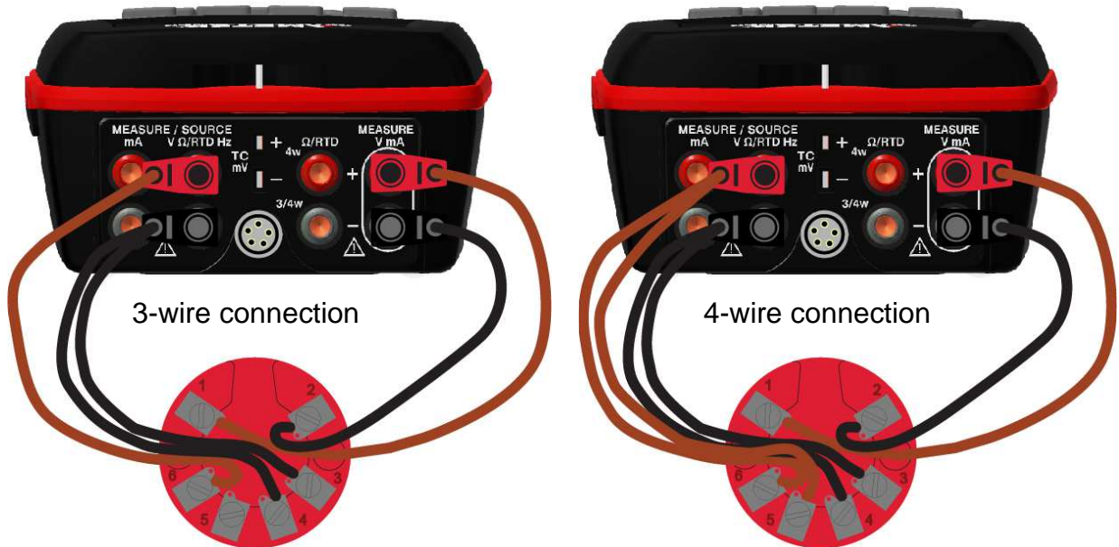
Figure 12 Using a 3- or 4-wire Connection for RTDs
