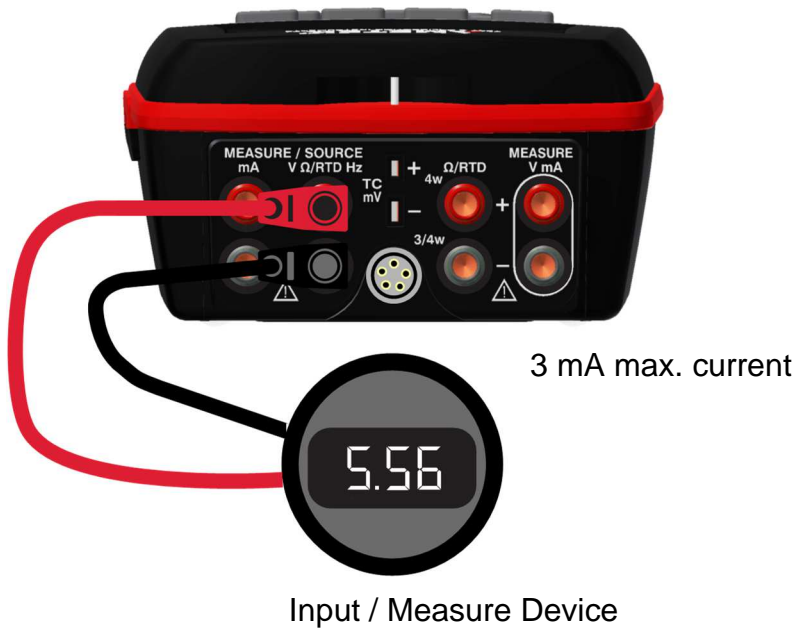
Figure 18 Connections for Testing an Output Device
